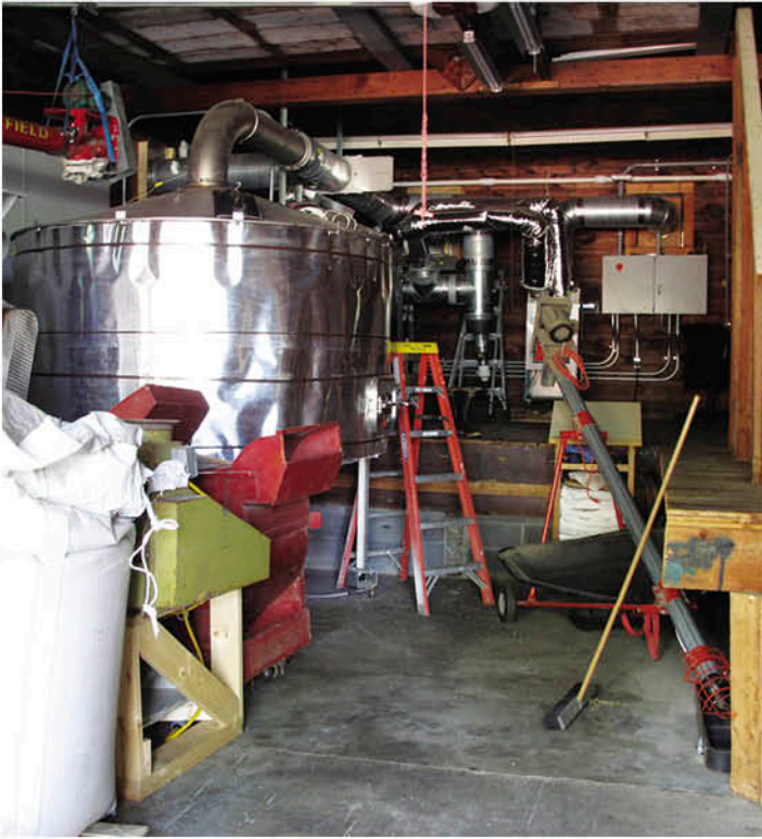
Above left Valley Malt’s first commercial prototype: a one-ton malting vessel designed and made by Christian Stanley.
